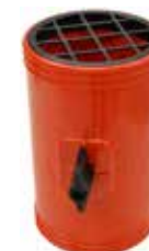
Heavy duty plastic cowling glass reinforced diam. 4" resistant up to 400°F equipped with butterfly valve and safety net.
