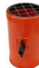
Heavy duty plastic cowling glass reinforced diam. 4" resistant up to 400°F equipped with butterfly valve and safety net.
