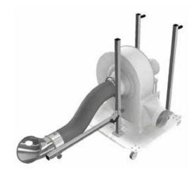
Heavy duty mobile exhaust extraction system with high pressure fan, tilting arm mounted stainless steel nozzle, all mounted on trolley with double handle and 4 castor wheels (2 locking). To be completed with expulsion hose GROLLY-GTP.
