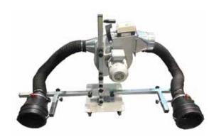
Portable extraction system with 0.5 Hp motor and a structure with 2 indipendent supporting arms equipped with two rubber nozzles for sports cars.
