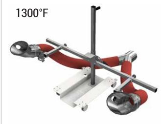
Trolley mounted nozzle for double exhaust pipes, two very high temperature resistant hoses 4' long each, clamps and two stainless steel nozzles mounted on indipendently adjustable armlets.
